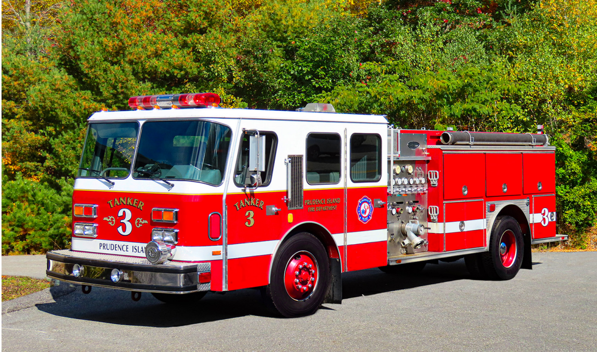
Tanker 3 1991 Emergency One 1,000-gallon capacity
