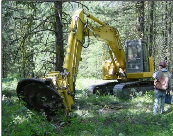
Figure 28: Excavator with mastication head Credit: US Forest Service
