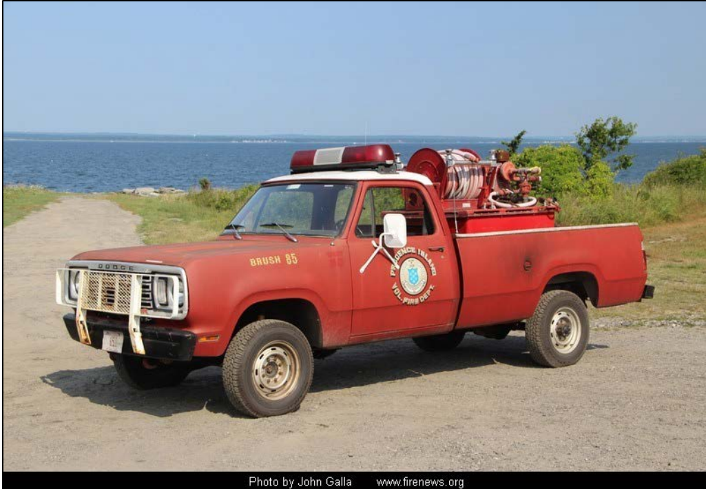
Figure 18: Brush #85 1977 Dodge 4x4 (off-road capable) 250-gallon capacity
